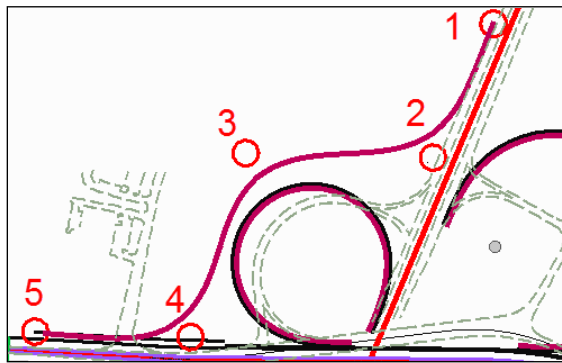
Five points used as P.I. for northwest ramp.
