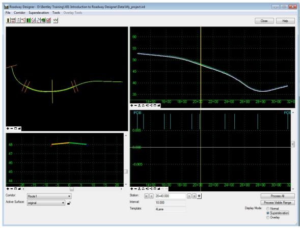
To set up super elevation we must first calculate the superelevation rates.
