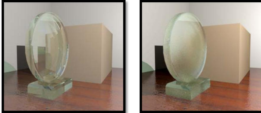
Transparent material with Blur Refractions disabled (left) and enabled (right)
