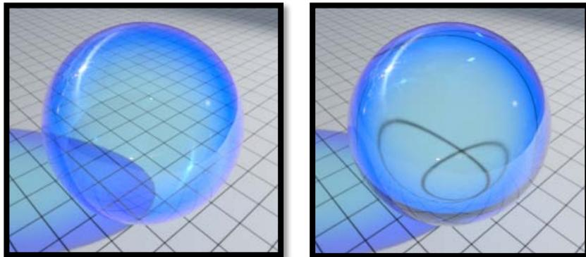
*Refraction options left, preview sphere with refract of 1.0(air) center and refract 1.474 right*
