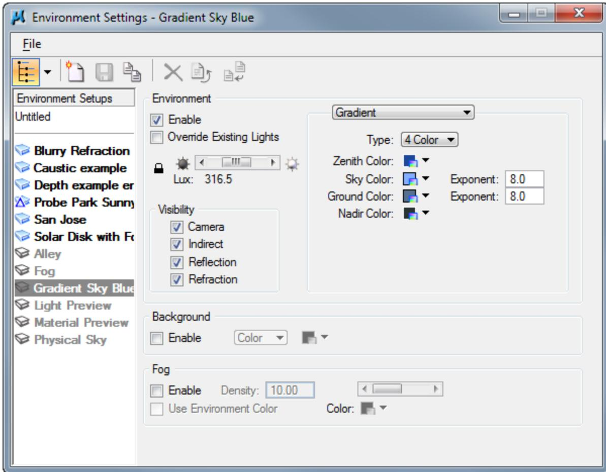
Environments can be saved and recalled at render time. The environments are similar to render settings in that they can be stored in a DGN library file (DGNLib). If you want to have environment setups that can be used by any instance of MicroStation, edit the `Luxology_render.dgnlib` or create a new library file and place it in a DGNLib search path with your custom environments.
